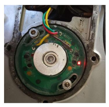
Now it is time to apply power to the Hall Advancer so we can observe the LEDS and set the timing up
