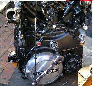
The next step is to install the rotor onto the rear of the crankshaft.
