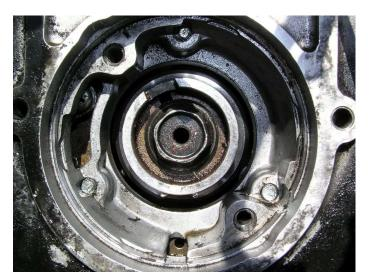
The next picture shows the crank access needed to be able to set the timing
