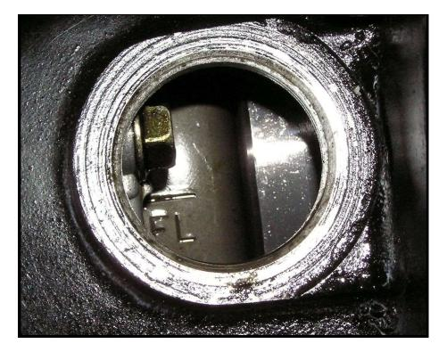
Loosen the M5 bolt(s) to adjust the timing –
