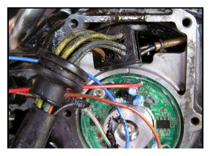
Position the wires out of the way of the spinning rotor and clear of sharp edges on the case.
