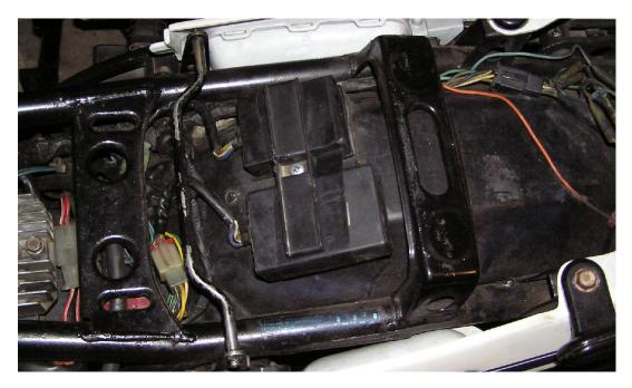
Original configuration : this shows a large and small box as fitted to the 83 vf750f,s,c. The 82 (which this bike is) actually has two of the smaller boxes seen at the top of the picture – The larger box has the addition of a rev limiter which was not present on the 82 models.
