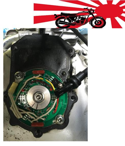
Now it is time to apply power to the Hall Advancer so we can observe the LEDS and set the timing up
