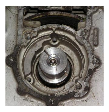
The next step is to put the hall pickup and advancer circuitry in place – The LEDS and wires face outward.
