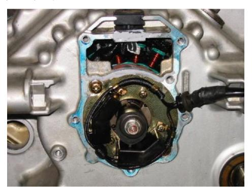
The original system has two pickup coils that contain a magnet and a wire coil. When the little bump on the rotor passes the pole face (the small metal bit in the middle of the black pickup) the magnetic flux through the coil changes due to the nearby presence of the steel rotor.
