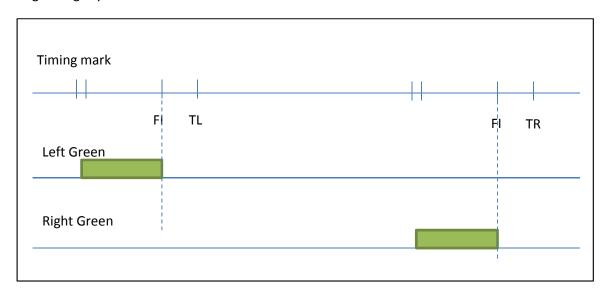
Rotate the engine and check that the turn ON of the Green LED occurs near the Full Advance marks – these are a pair of lines || before the FI LEFT and FI RIGHT marks that indicate the stock full advance range.
