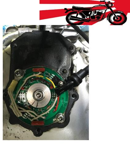
The rotor is in a fixed location so it is necessary to rotate the Hall Advancer circuit to achieve the required timing result.
