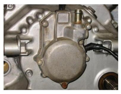
Position the wires out of the way of the spinning rotor and clear of sharp edges on the case and install the rear cover.
