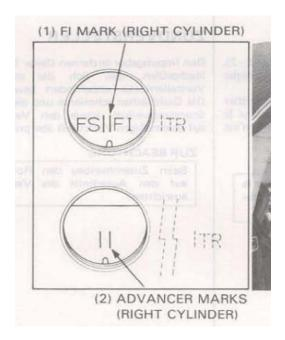
• Loosen the M5 bolt(s) to adjust the timing –
