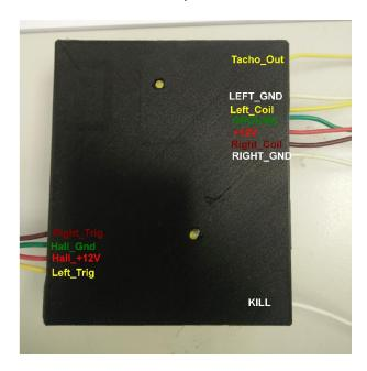
This needs to mount somewhere near where the NEC igniter modules were placed or under the seat (space permitting).
