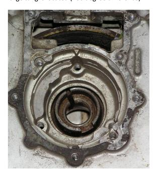
The next picture shows the crank access needed to be able to set the timing
